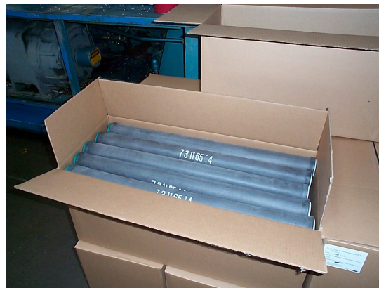
Figure 8: Fine Bubble Diffusers
