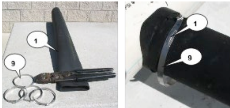
Figure 11: Image of Membrane with Clamp Installed
