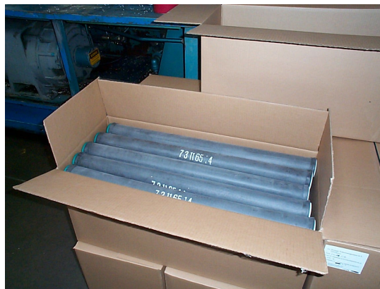
Figure 8: Fine Bubble Diffusers
